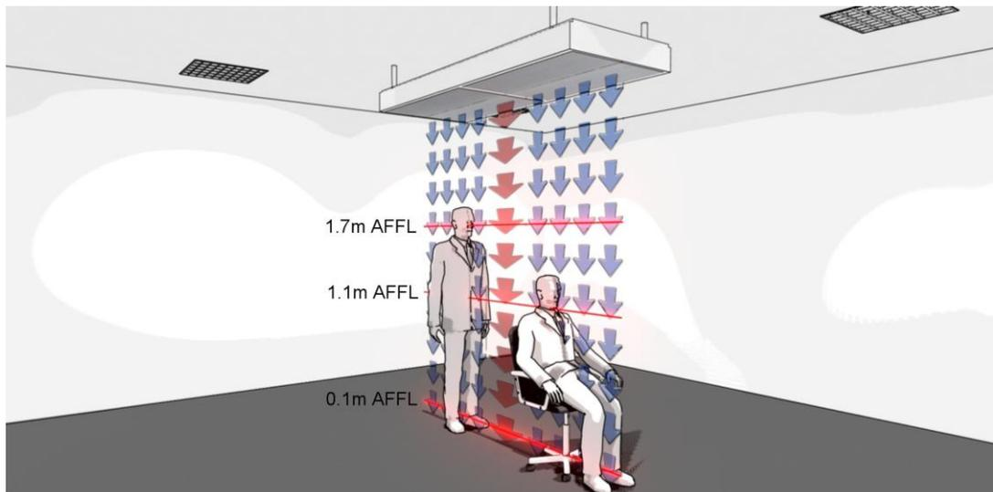
**Fig 4. Typical Passive Chilled Beam System**
