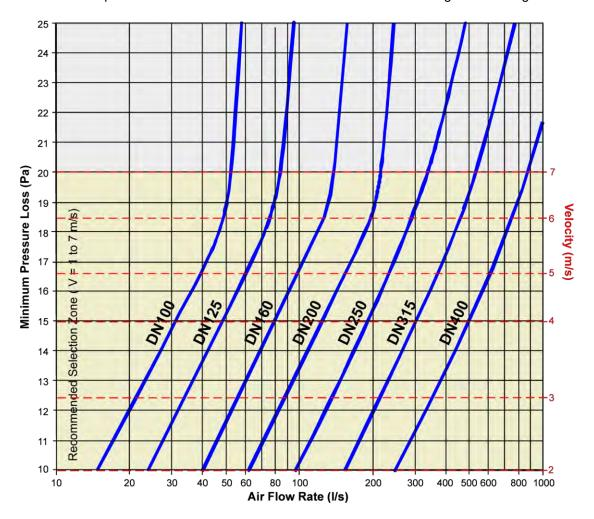
To ensure best practice selection, for controllability and noise we recommend that the VAV type RND selection should ensure a design velocity of between 1.0 and 7.0 m/s at the design flow rate.
