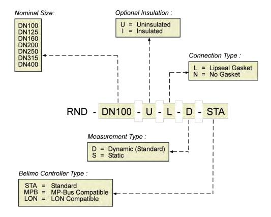
At time of order please specify the required minimum and maximum flowrates (Vmin, Vmax) to enable factory setting; failure to provide the specification at time of order will result in units being delivered based on Vmin = 0, Vmax = See Table page 2.
